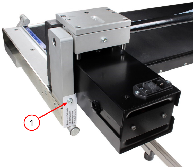
Figure 34 Remove transport screw and plastic ring VARGA VA 21-15 and VA 31-15
