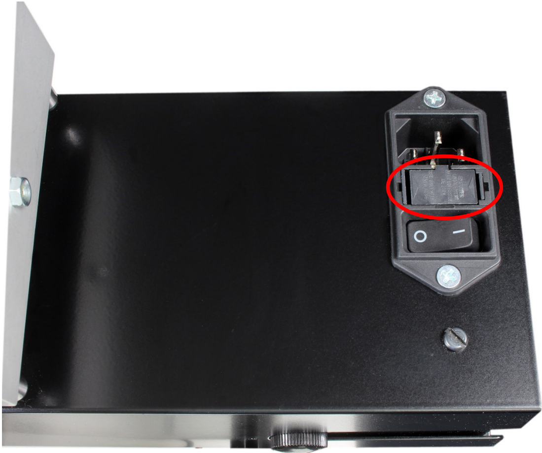
Figure 52 Replacing a fuse
