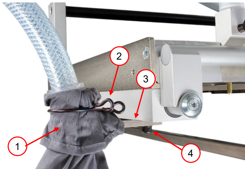
Figure 25 Fitting the VARGA VA 11 chip bag
