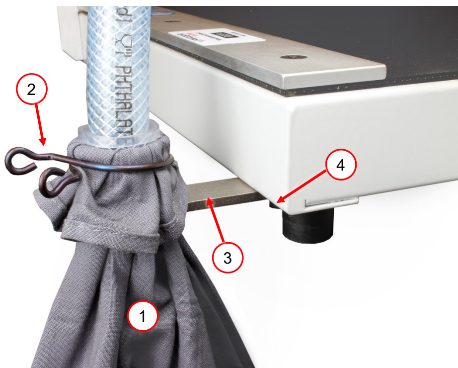
Figure 21 Fitting the VARGA VA 10 chip bag
