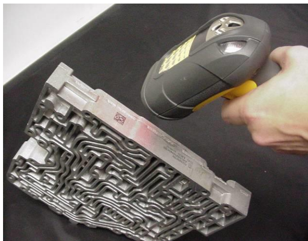
Data Matrix on Aluminum Auto Part
