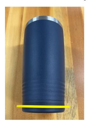
• Place the tumbler with attached elevation spacer onto the rollers of the rotary attachment.
